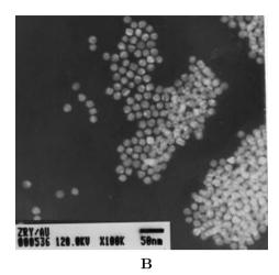
Fig. 4 TEM images of gold nanoparticles (A) and oligonucleotide-modified gold nanoparticles (B).
